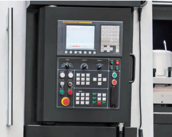
• Swing control pendant, Remote MPG, convenience for the operator.
